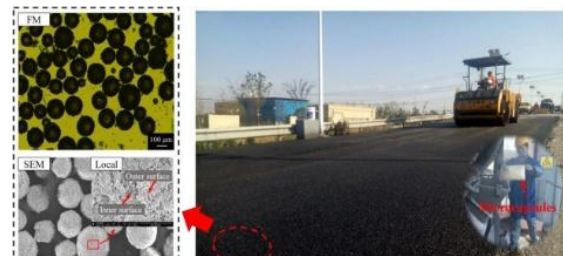
Figure 12 Illustration of the Self-Healing Mechanism in Asphalt Using Microcapsules [42]
