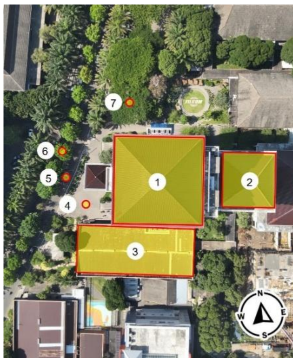
Figure 4. The points and areas of surface temperature surrounding the building
