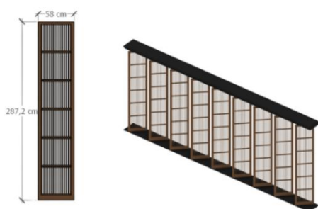
Figure 11. Dimensions of the Timber Louvered Secondary Skin Panels in the Proposed Design for the Phase II SD Labschool UPI Building.
